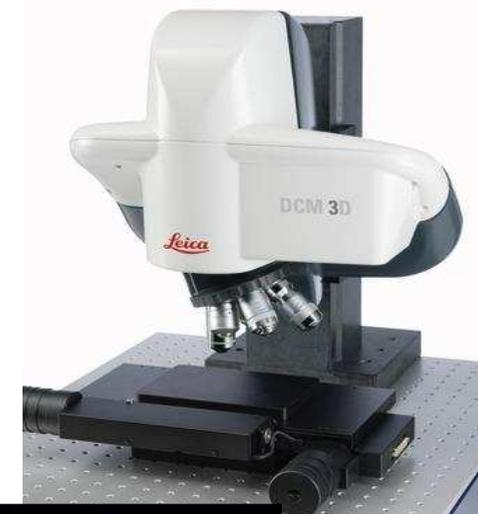
**Interferometro-Confocale Leica DCM3D**
